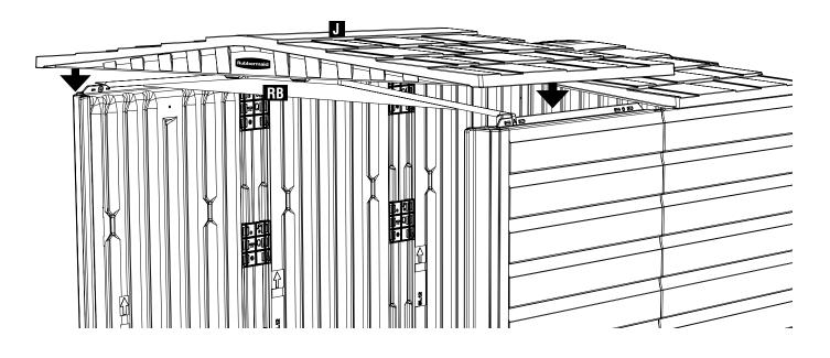
Slightly raise front edge of roof enough to allow positioning of **Roof Brace (RB)** onto the side walls as shown. Lower the roof onto the walls and align **Roof Brace (RB)** into pocket in **Front Roof (J)**.
